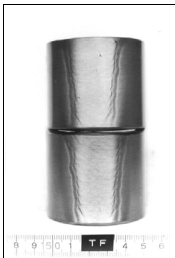
Fig. 6.4 — Side bend specimens after test
