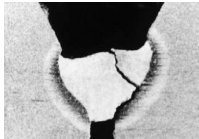
(F) Root crack
