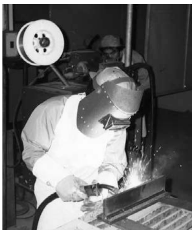
Fig. 4.26 — Typical protective clothing in gas shielded metal arc welding
