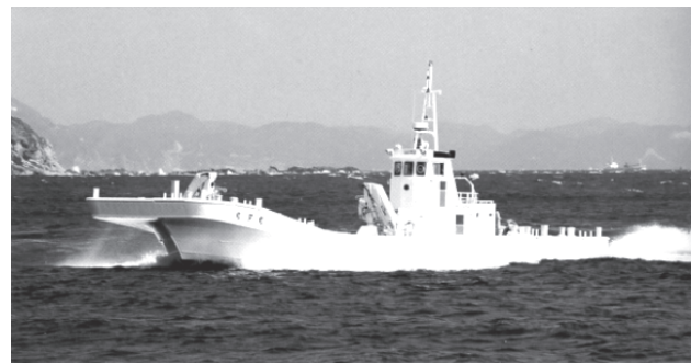
Photo 1.2 A fishing boat made of aluminum alloy structural components. (Source: Kobe Steel's brochure)
