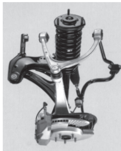
Photo 1.4 Forgings and castings of aluminum alloy for automobile components (Source: Kobe Steel's brochure)
