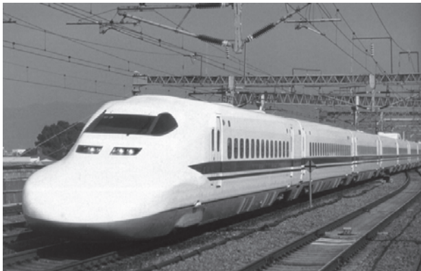
Photo 1.1 Shinkansen high-speed trains uses plates, extrusions, castings and forgings of aluminum alloy (Source: Kobe Steel's brochure)
