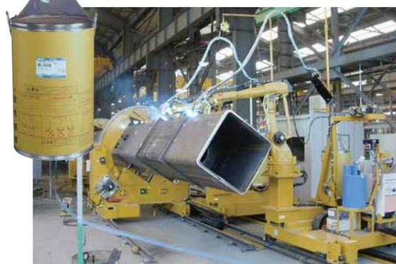
15 Система сварки / Welding System for building structure
