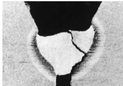
(F) Root crack
