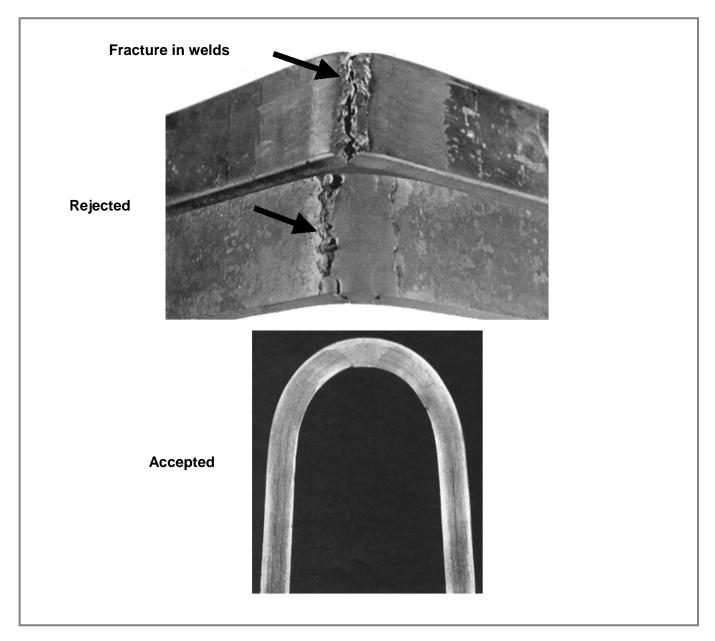
Fig. A-1 Fracture in welds caused by weld imperfections (Bend test results of weld joints)
