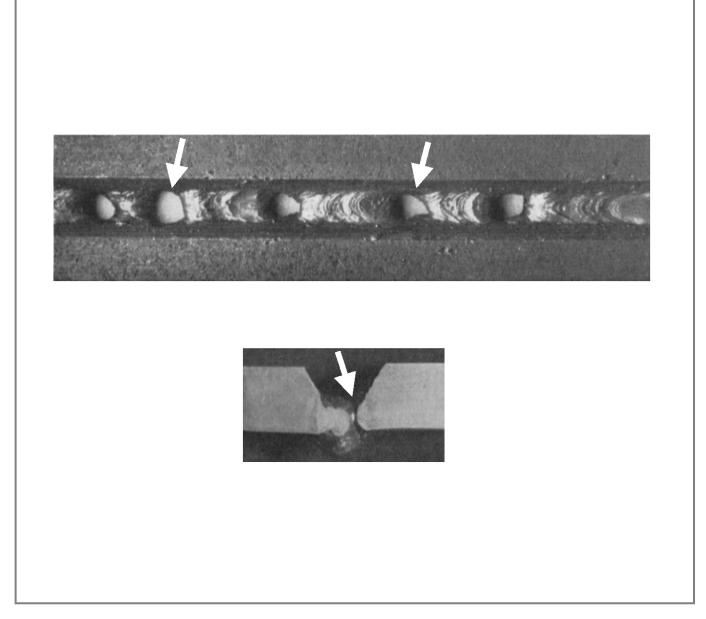
Fig. 14 EXCESSIVE MELT-THROUGH (BURN-THROUGH)
