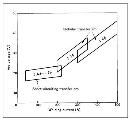
Fig. 3-10 — A general guidance to proper ranges of welding current and arc voltage for globular and short-circuiting transfer arcs with solid wires of 0.6, 1.2, and 1.6mm  $\phi$
