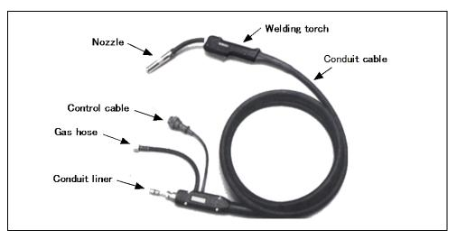
Fig. 3-21 A conduit liner should be taken out periodically from the conduit cable, and check its appearance to ensure good wire feedability
