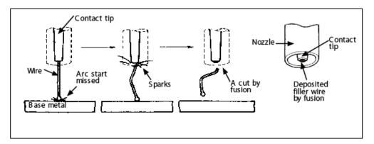
Fig. 3-15 A process of burn-back in GSMAW
