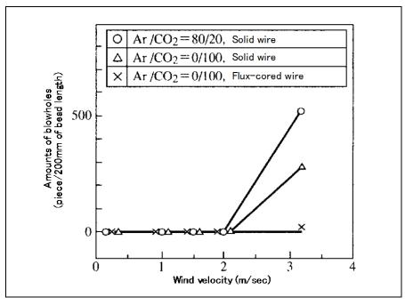
Fig. 3-16 Effects of wind on amounts of blowholes in GSMAW (Wire size: 1.2mm  $\phi$ , Welding current: 300A, Shielding gas flow rate: 25
