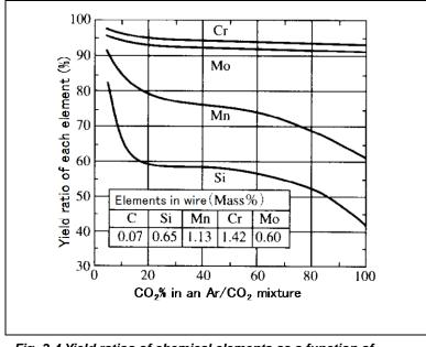
Fig. 3-4 Yield ratios of chemical elements as a function of  $CO_2\%$  in an Ar/CO<sub>2</sub> mixture
