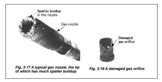
In addition, a loose connection and tear in the gas passage can leak pressurized shielding gases, thereby causing lack of shielding even when the gas regulator indicates the correct pressure and the gas flow meter shows the correct flow rate. In order to prevent this trouble routine maintenance is important.
