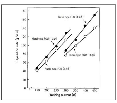
Fig. 3-5 A comparison between rutile- and metal-type FCWs on deposition rate in  $CO_2$  GSMAW (wire extension: 25mm)
