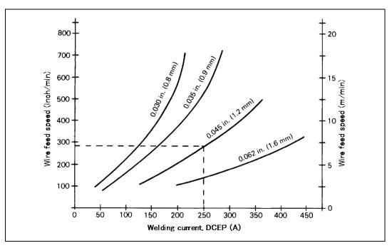
Fig. 3-1 Typical welding currents vs. wire feed speeds for carbon steel electrode (Source: AWS Welding Handbook)
