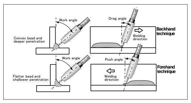
Fig. 3-23 Definitions of work angle, drag angle, and push angle
