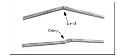
Fig. 3-22 A bend and crimp cause irregular wire feeding and an unstable arc
