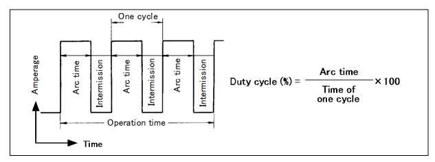
Fig. 3-2 A definition of duty cycle
