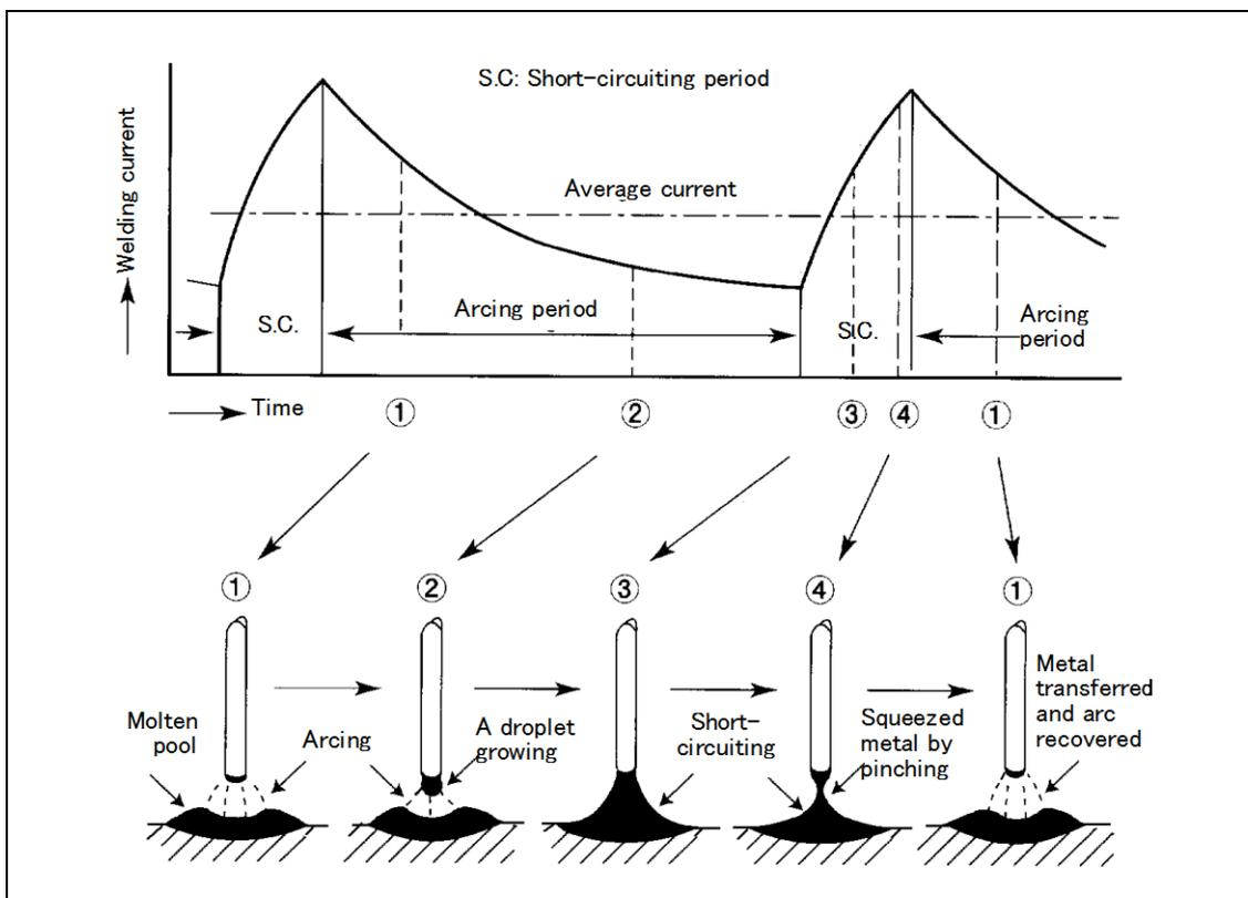
**Fig. 3-7 — The mechanism of typical short-circuiting droplet transfer associated with welding current output**
