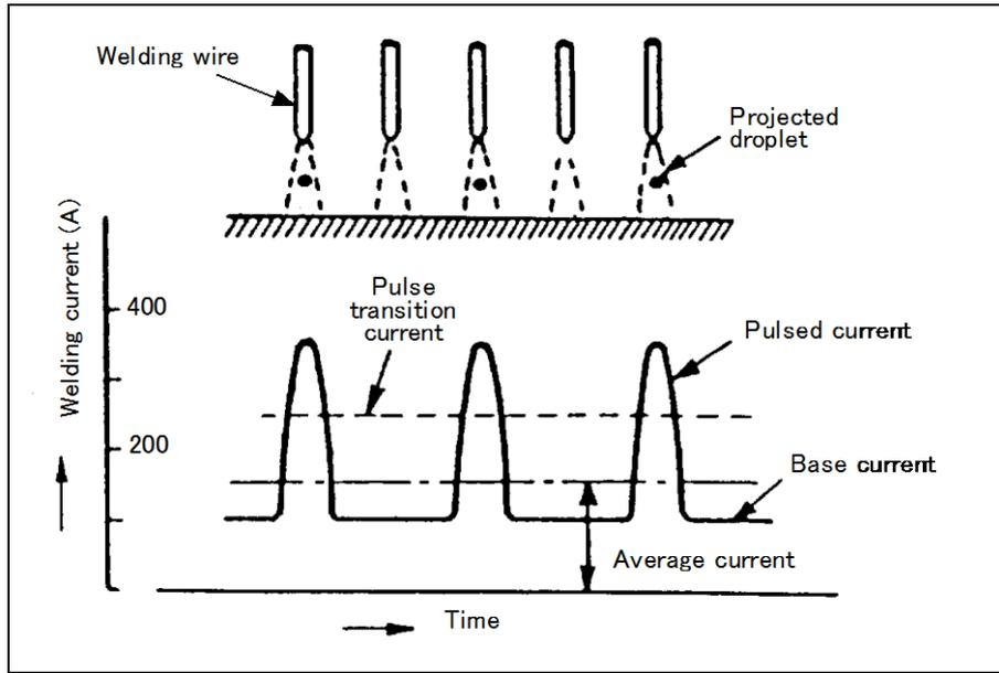
Fig. 3-11 Typical pulsed-arc metal transfer (For solid wires)
