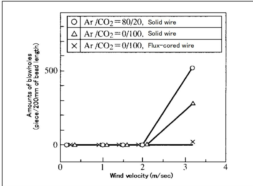
**Fig. 3-16 Effects of wind on amounts of blowholes in GMAW**
