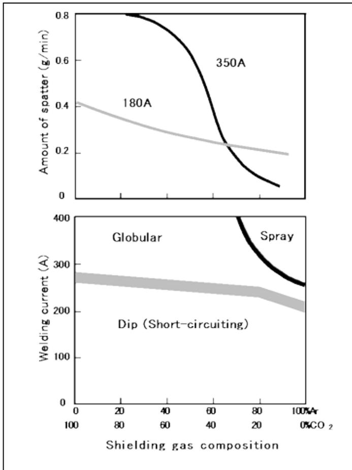
**Fig. 3-8 Droplet transfer modes and the amount of spatter in conventional GMAW using a solid wire**
