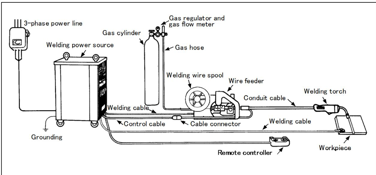
**Fig. 1-1 Typical arrangement of the gas shielded metal arc welding process**
