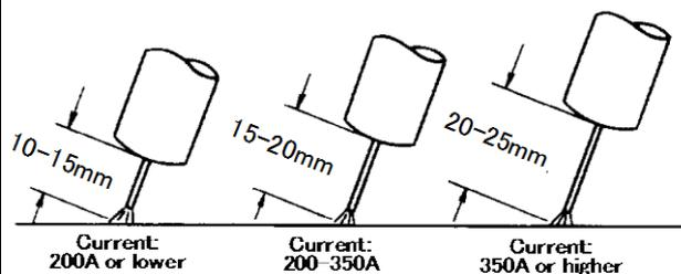
**Fig. 2-12 Proper nozzle-to-work distance depends on welding currents.**
