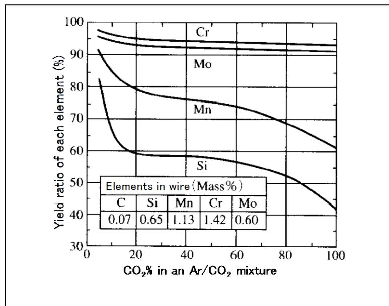
**Fig. 3-4 Yield ratios of chemical elements as a function of CO<sub>2</sub>% in an Ar/CO<sub>2</sub> mixture**
