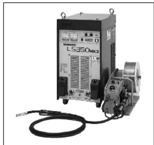
**Fig. 1-2 A set of welding power source, wire feeder, and welding torch**
