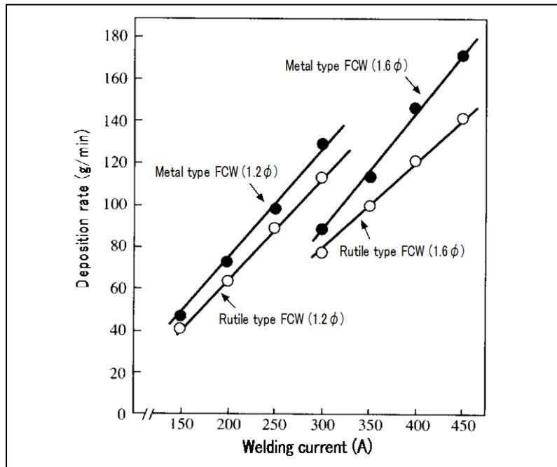
**Fig. 3-5 A comparison between rutile- and metal-type FCWs on deposition rate in CO<sub>2</sub> GSAW (wire extension: 25mm)**
