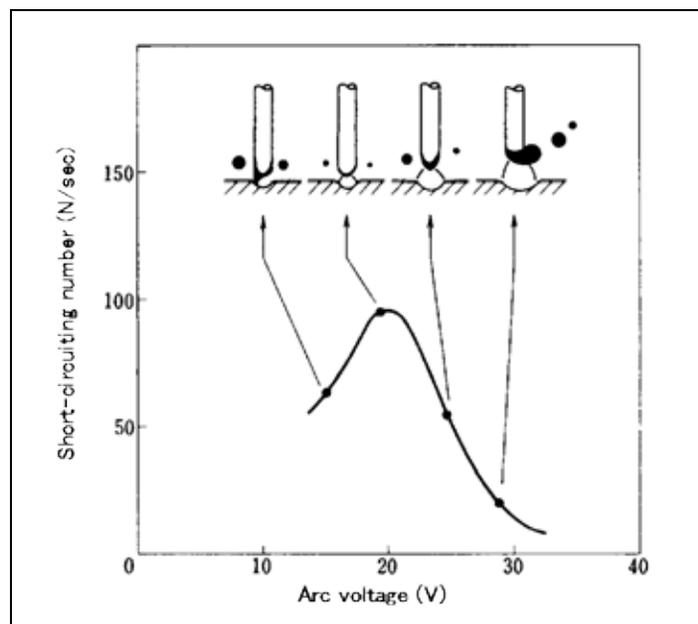
**Figure 3-10** shows a general guidance to proper ranges of welding currents and arc voltages in the cases of globular and short-circuiting arcs; more fine adjustment may be needed for an exact solid wire to be used.
