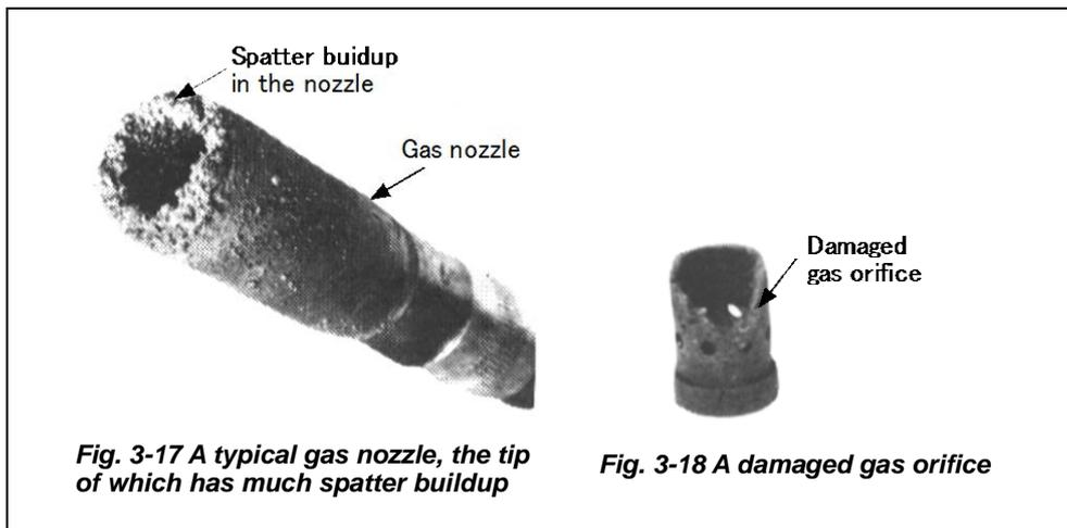
**Fig. 3-17 A typical gas nozzle, the tip of which has much spatter buildup**
