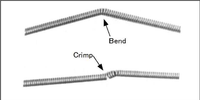
**Fig. 3-22** A bend and crimp cause irregular wire feeding and an unstable arc
