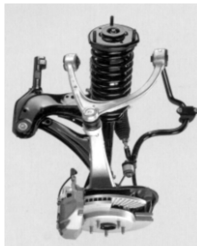
Photo 1.4 Forgings and castings of aluminum alloy for automobile components (Source: Kobe Steel's brochure)
