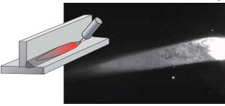
In gas-shielded arc welding, it is important for the welding wire (consumable electrode) to melt and transfer consistently to the weld pool. The precise observation of the arc phenomena can provide a lot of information useful for the development of a welding consumable. In recent years, the behaviors of molten metal and slag have become possible to observe in high accuracy, even in the horizontal fillet and vertical upward welding.
