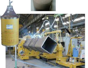
Система сварки / Welding System for building structure
