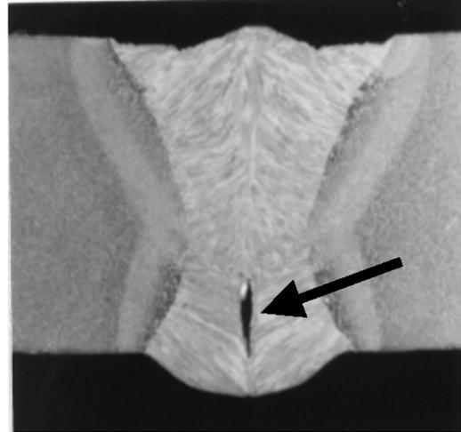
**Longitudinal crack in SMAW**
