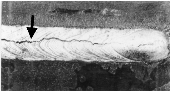
**Sulfur crack in SMAW**
