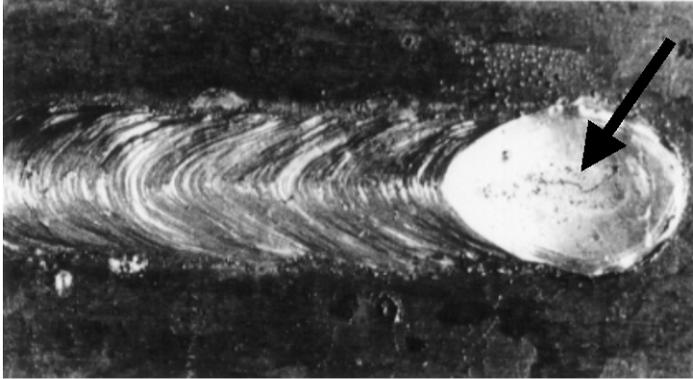
**Pear-shape crack in SAW**
